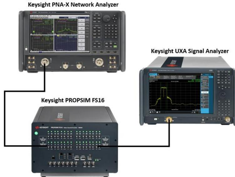
FIGURE 13. MEASUREMENT SETUP FOR VALIDATING DOPPLER SPECTRUM AND TEMPORAL CORRELATION.
