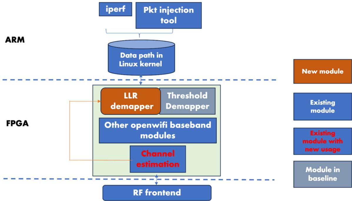
FIGURE 18. POC ARCHITECTURE OF JAMMER RESILIENT PHY ON OPENWIFI.
