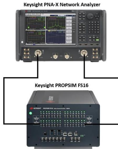
FIGURE 11. MEASUREMENT SETUP FOR VALIDATING INSERTION DELAY AND POWER DELAY PROFILE (PDP).
