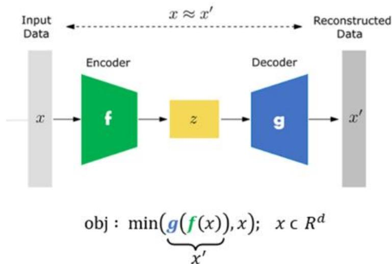
FIGURE 25. ILLUSTRATION OF AUTOENCODER USING MAIN BLOCKS AND OBJECTIVE FUNCTION.
