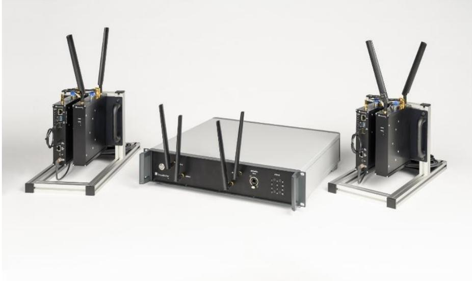
**FIGURE 19. UWIN SETUP WITH ONE BASE STATION AND TWO FIELD DEVICES OF THE WIRELESS COMMUNICATION SYSTEM.**
