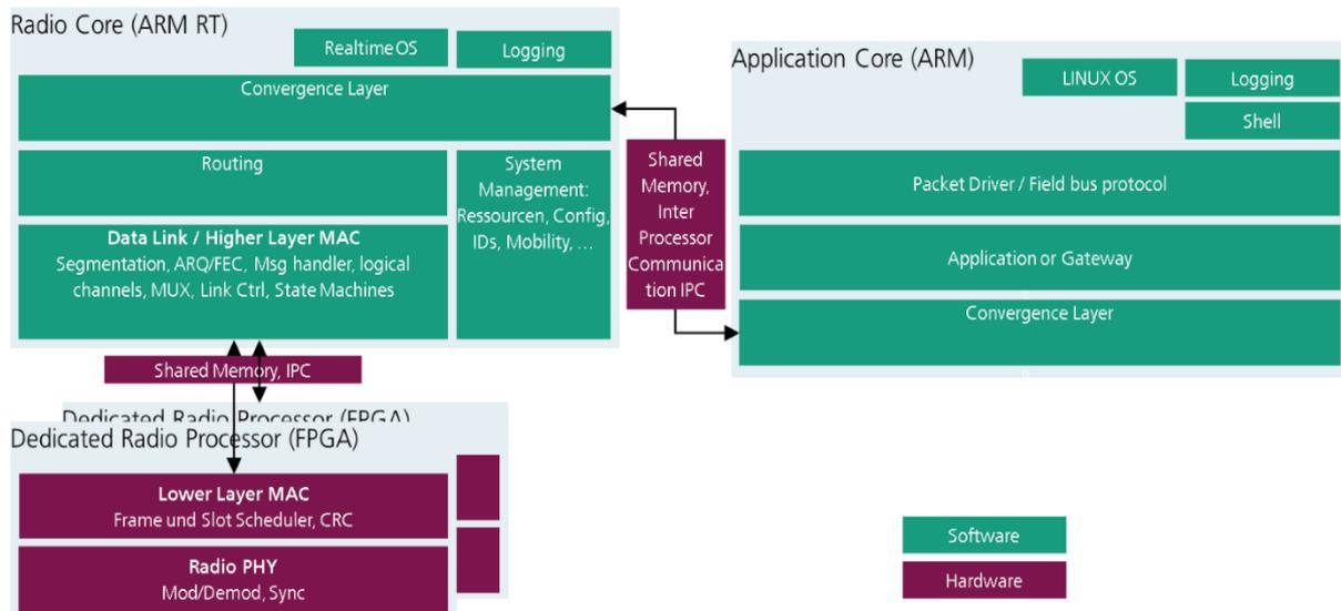
FIGURE 20. SYSTEM ARCHITECTURE OF THE UWIN WIRELESS NODES.
