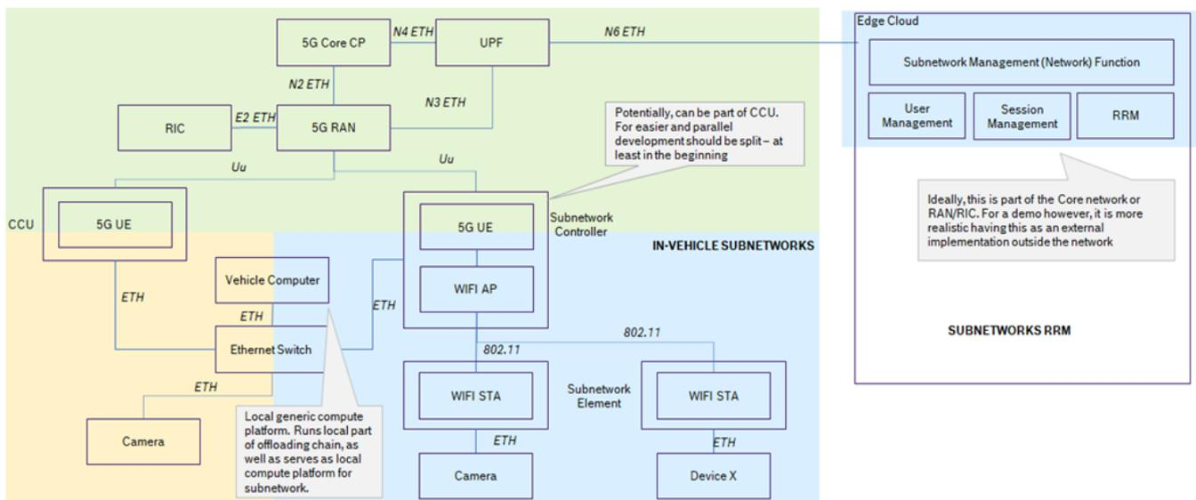
FIGURE 22. MAIN BUILDING BLOCKS ENABLING THE PoC DEVELOPMENT.
