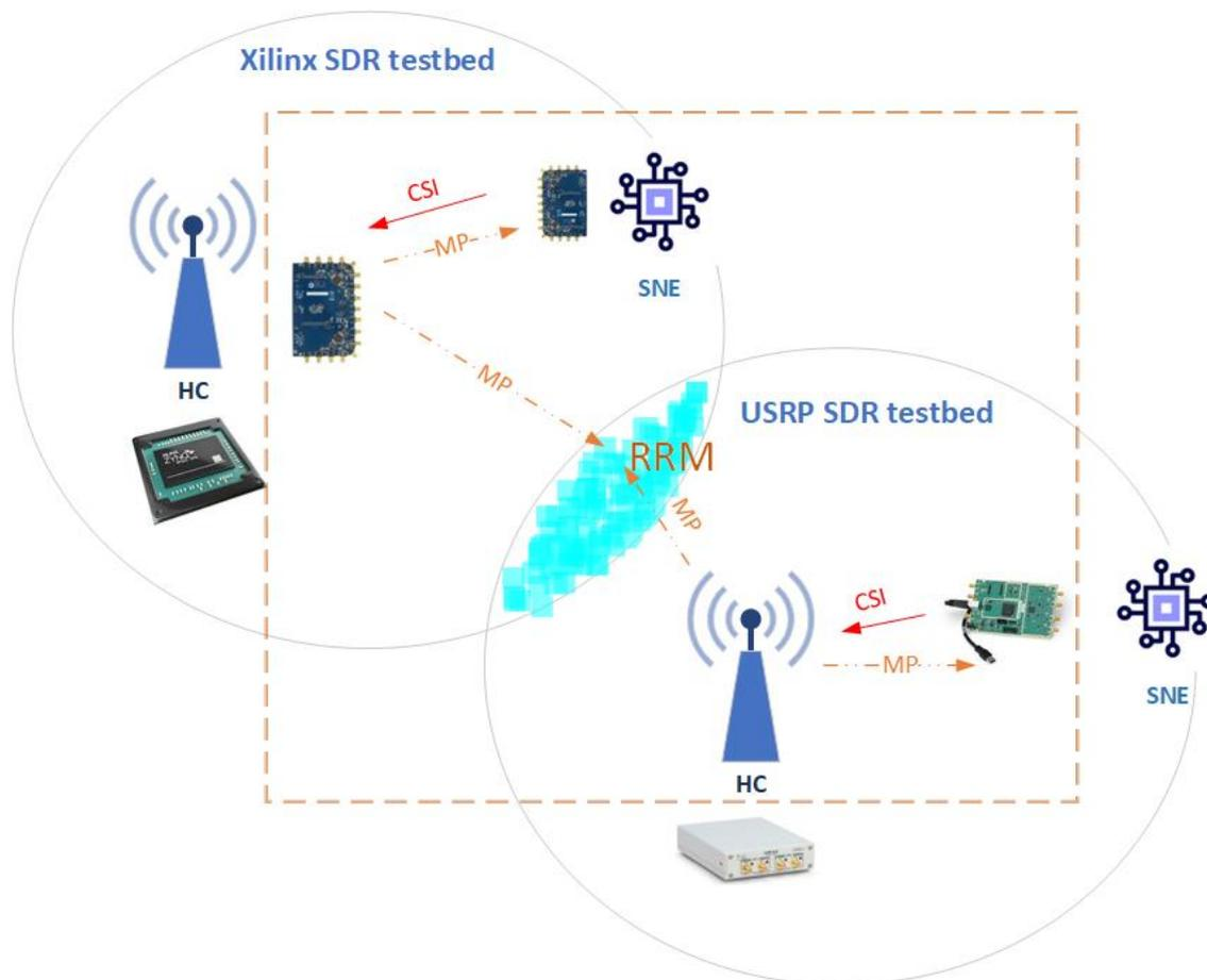
FIGURE 24. PoC SETUP FOR THE CENTRALIZED/DISTRIBUTED INTERFERENCE MANAGEMENT.
