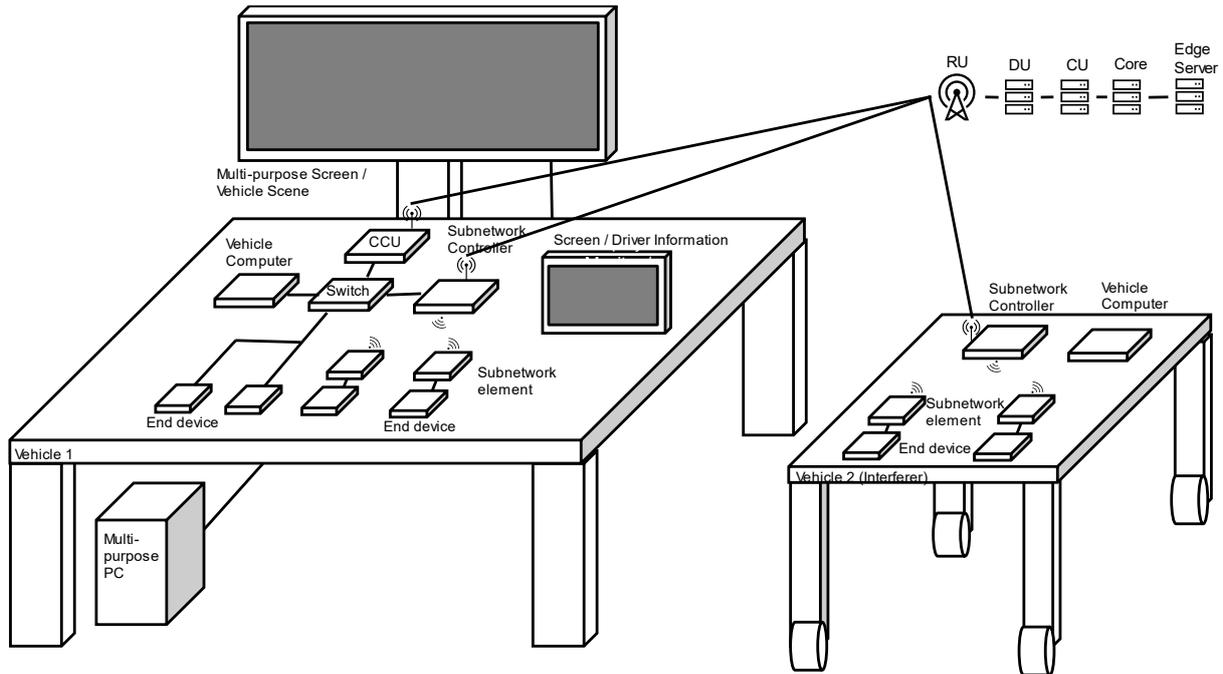
FIGURE 23. CENTRAL RADIO RESOURCE MANAGEMENT BETWEEN IN-VEHICLE NETWORKS.
