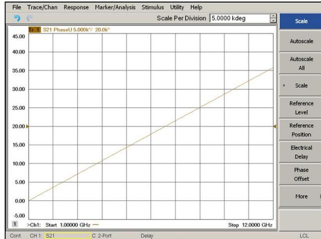
FIGURE 12. EXAMPLE UNWRAPPED PHASE TRACE OF DUT ELECTRICAL DELAY.
