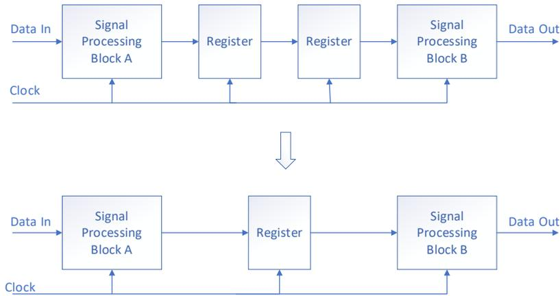
FIGURE 4. REMOVING UNNECESSARY LOGIC FROM THE CRITICAL PATH.
