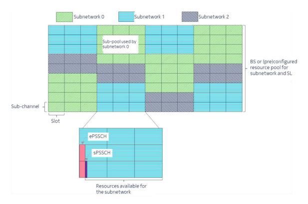
FIGURE 16: EXAMPLE OF SUB-POOL RESOURCES RESERVATION BASED ON EPSCCH AND SPSCCH.
