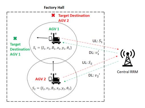
FIGURE 13: ILLUSTRATION OF THE MULTI-AGV SUBNETWORK JOINT NETWORK-CONTROL PROBLEM. EACH AGV CONTAINING A SUBNETWORK AND PHYSICALLY MOVING TO A PREDEFINED GOAL DESTINATION.
