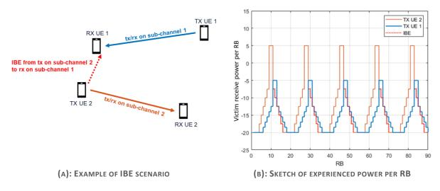
FIGURE 19: EXAMPLE SCENARIO WHERE IBE ISSUES MAY OCCUR (A) AND SPECTRUM POWER SEEN FROM RX UE (B)
