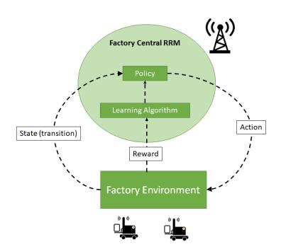
FIGURE 14: THE GENERAL FRAMING OF THE AGV SUBNETWORK CONTROL PROBLEM.
