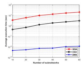
FIGURE 8: COMPUTATIONAL RUNTIME FOR DIFFERENT ALGORITHMS
