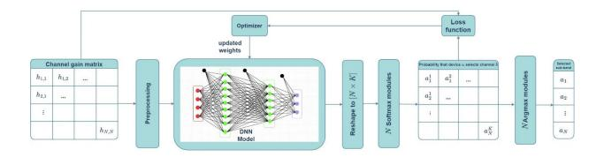
FIGURE 3: STRUCTURE OF THE PROPOSED DNN MODEL
