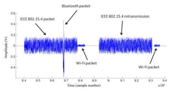
FIGURE 30: COEXISTENCE OF TECHNOLOGIES IN THE 2.4-GHZ BAND. MEASUREMENTS MADE BY THE NATIONAL INSTRUMENTS USRP [33]
