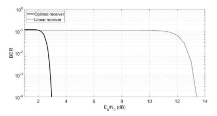
FIGURE 33: EFFECT OF MISMATCH DECODING, WHERE THE LINEAR RECEIVER IS USED IN AN IMPULSIVE ENVIRONMENT.
