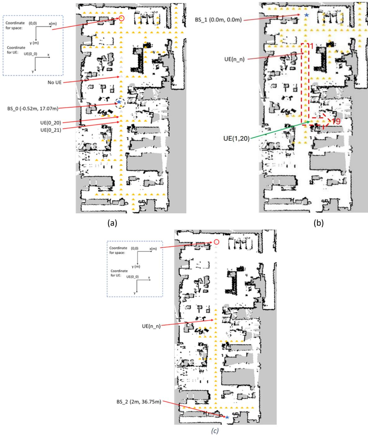
Figure 4. Measurement map for (a) Rx\_0, (b) Rx\_1 and (c) Rx\_2, where the Rx and the Tx are denoted by BS and UE, respectively. Note that Rx locations are noted by blue stars and those of Tx by yellow triangulars.
