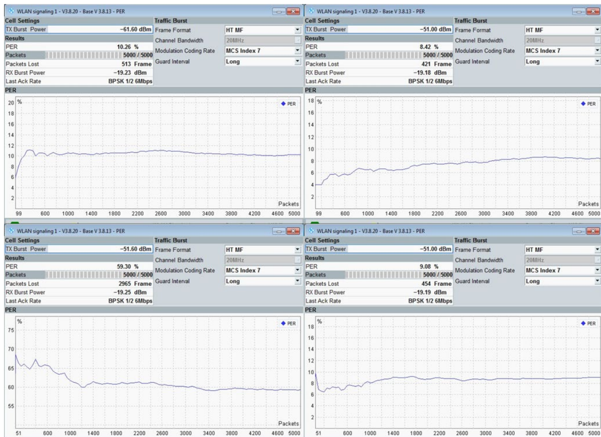
FIGURE 32. IMPACT OF WIDEBAND JAMMER IN TERMS OF RX SENSITIVITY.
