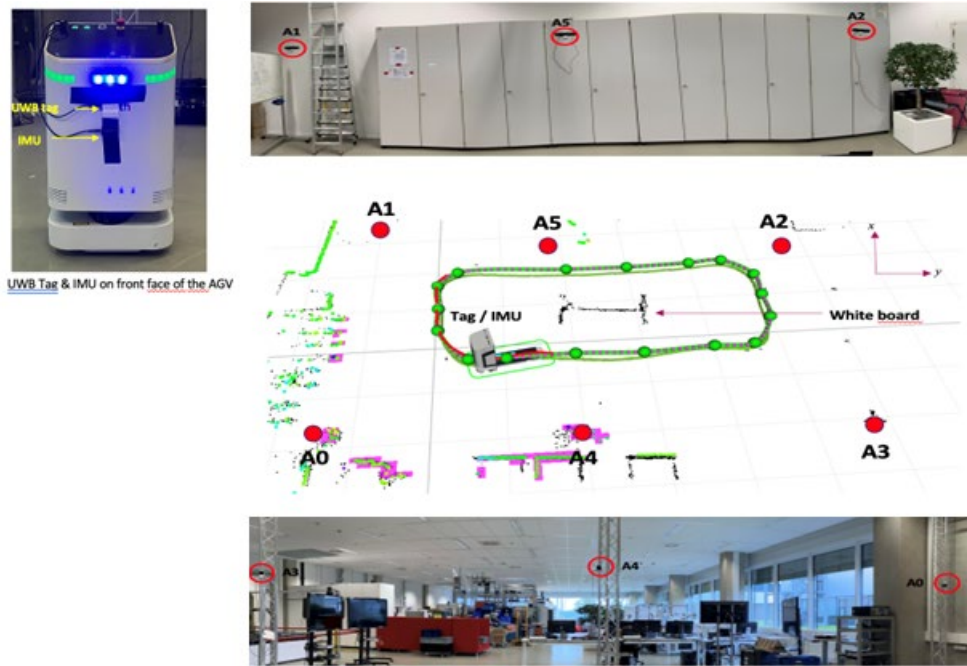
FIGURE 43. INDOOR POSITIONING ALGORITHM DEVELOPED FOR INDOOR SCENARIOS WHEN MANAGING IN-X SUBNETWORKS.
