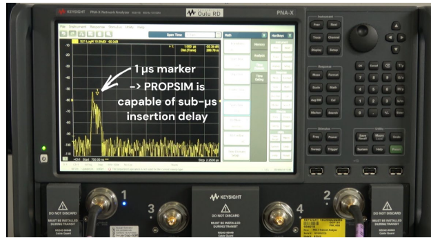
FIGURE 9. INSERTION DELAY MEASUREMENTS FOR THE IMPLEMENTED CHANNEL MODEL
