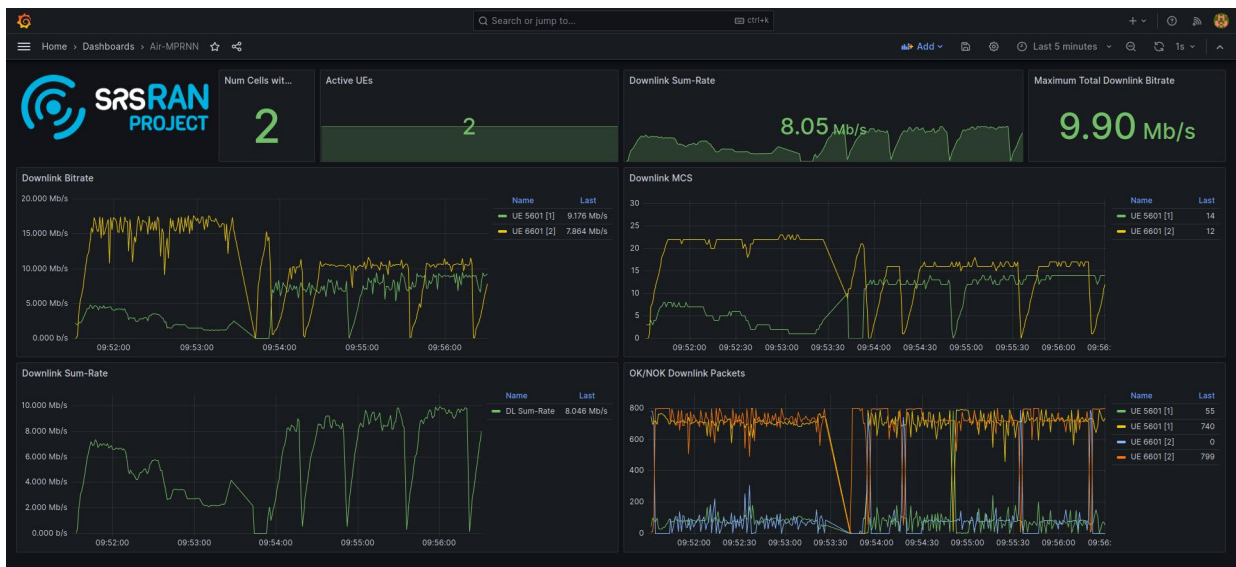
FIGURE 55. GRAFANA WEBUI DISPLAYING PLOTS OF DOWNLINK STATISTICS.
