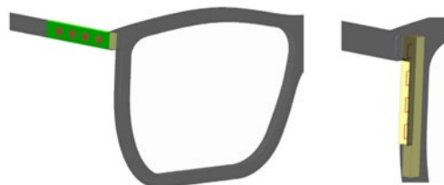
FIGURE 9. POSSIBLE PLACEMENT OF ANTENNA ARRAYS ON XR GLASSES. PICTURE FROM [7].
