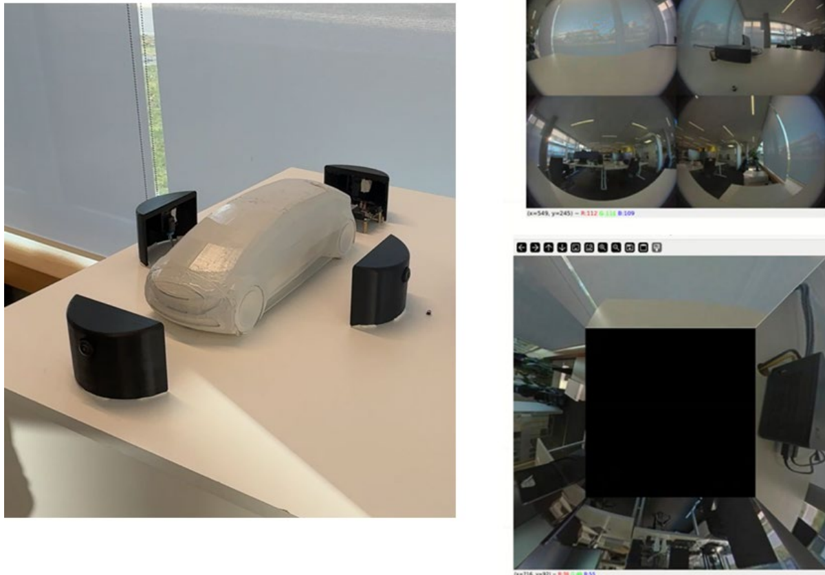
FIGURE 28. SURROUND VIEW CAMERA SYSTEM USING STITCHING ALGORITHM.
